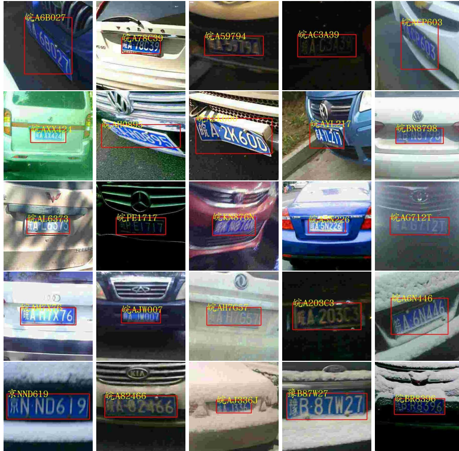
Fig. 4. Detection and recognition results on CCPD with our RPnet model. Each image is the smaller license plate area extracted from the original resolution 720 (Width) \times 1160 (Height) \times 3 (Channels).
