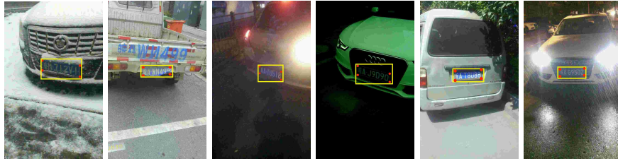
Fig. 1. Sample images from CCPD. Each image above is labelled with its bounding box (the yellow border) and four vertices location (four red dots). Other annotations are omitted here for simplicity.
