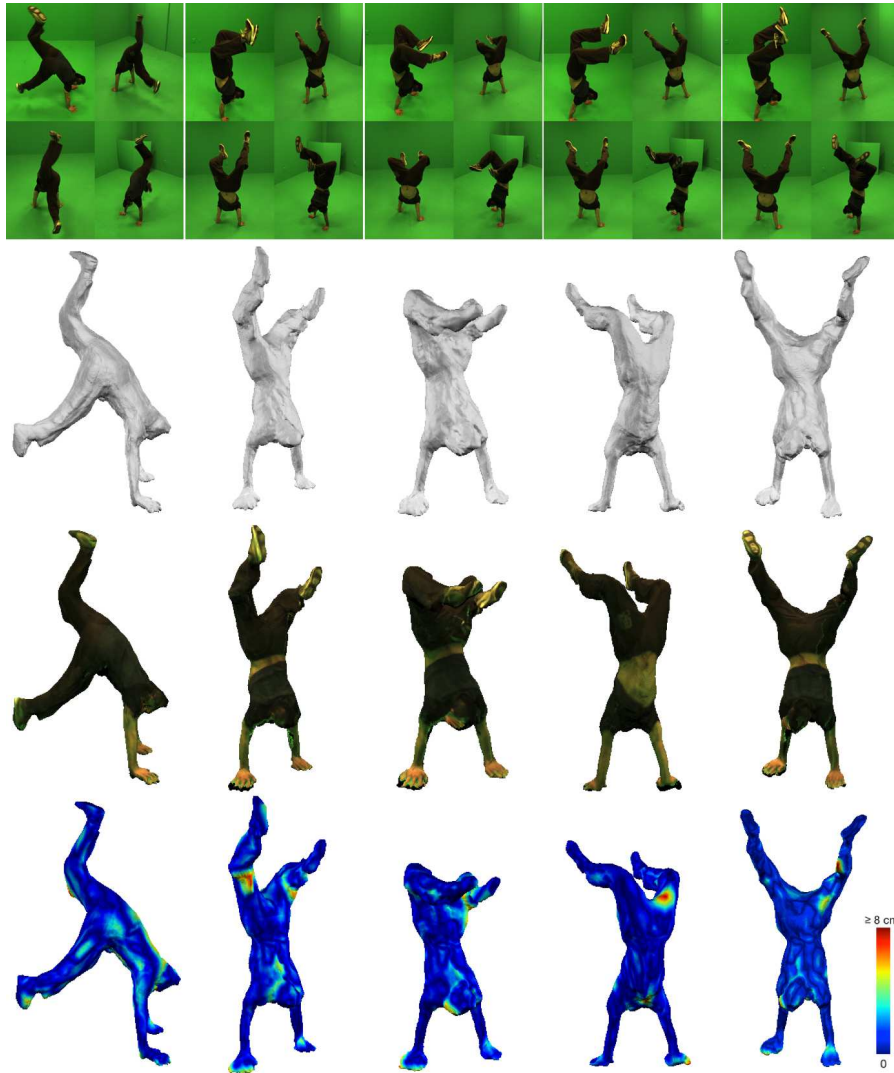
Fig. 4: Sequence results. Top to bottom rows: multi-view images, reconstructed mesh, textured mesh, and error visualization. From left to right, median mesh-to-scan distance: 0.94cm, 0.86cm, 0.82cm, 0.76cm, 0.85cm; mean mesh-to-scan distance: 1.31cm, 1.27cm, 1.21cm, 1.06cm, 1.25cm
