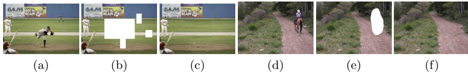
Fig. 6. Arbitrary shape inpainting of real-world photography. (a), (d): Input. (b), (e): Inpainting mask. (c), (f): Output.
