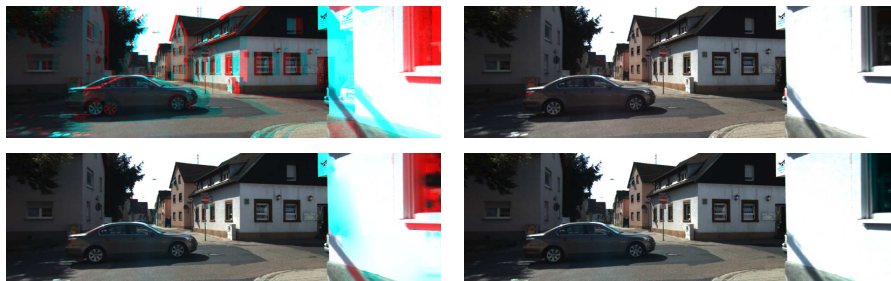
Fig. 6. Qualitative image separation results on the KITTI-2015 dataset. Top to bottom: Input, ground truth, result from Williém et.al. [8], our result. Our method successfully recovers the correct color of the large textureless region on the right of the image while the other method fails.
