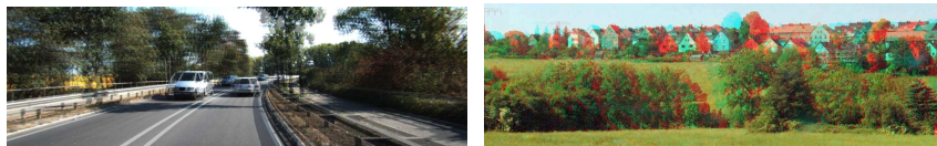
Fig. 1. Examples of image separation for single image based stereo computation. Left column: A double-vision image is displayed here. Right column: A red-cyan stereo image contains channels from the left and right images.
