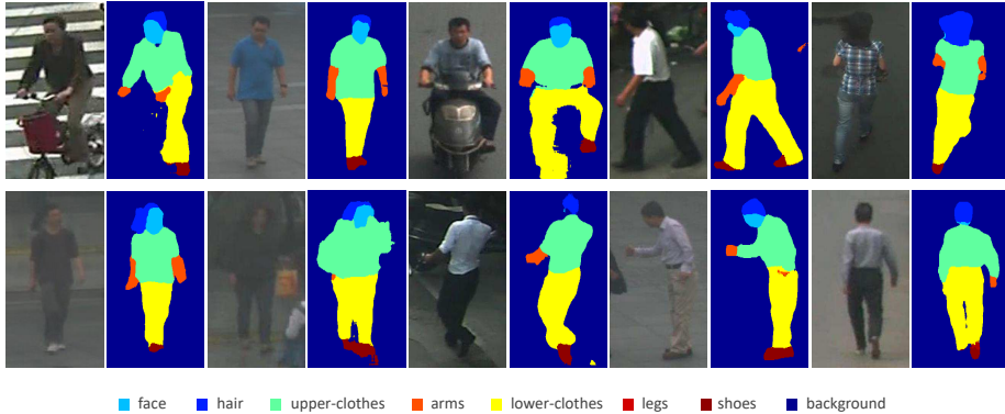
Fig. 6: Qualitative parsing results on the PPSS dataset. RGB image and the label map are showed in pairs.
