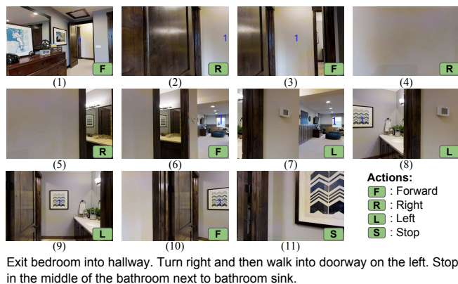
Fig. 6: An example trajectory executed by our RPA agent. Given the instruction and the starting position (1), the agent produces one action per time step. In this example we show all the 11 steps of this trajectory.
