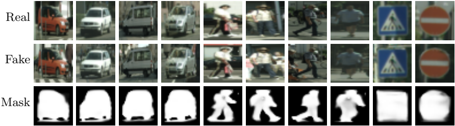
Fig. 7. Examples of Cityscapes images and masks generated by our method. The top row shows the original image, and the middle row is the fake generated by compositing onto a random background with the inferred mask (bottom row).
