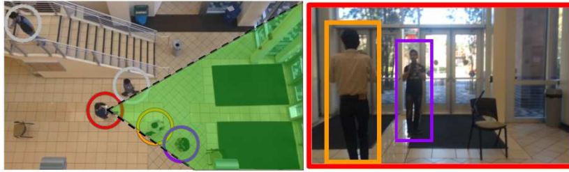
Fig. 1: A pair of top- (left) and egocentric (right) views. Self identification is to identify the egocentric camera holder (shown in red). Human re-identification is to identify people visible in the egocentric video, in the content of the top-view video (orange and purple).
