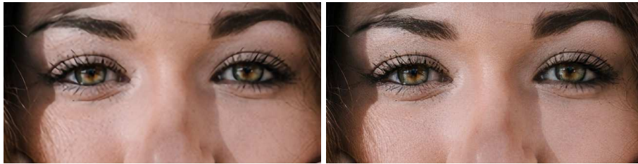
Fig. 1. Our SR results. The final result from our network trained with GAN (right) is much more perceptually realistic than the result obtained by our network trained with MSE only (left).
