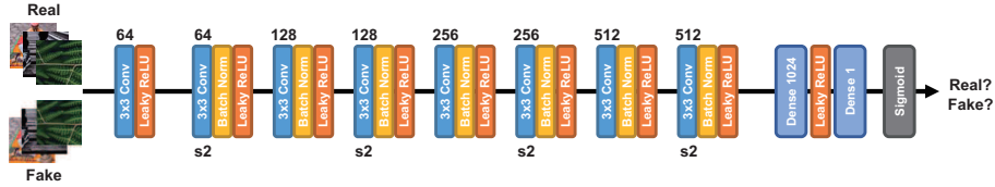
Fig. 3. Architecture of our discriminator network. The number above a convolution layer represents the number of filters, while s2 below represents the stride of 2.
