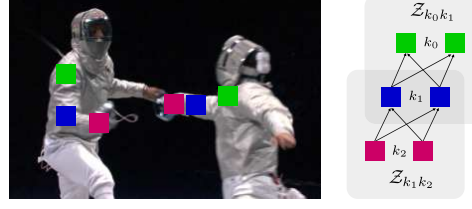
Fig. 4. Parts association defined as bipartite matching sub-problems. Matchings are decomposed and solved for every pair of detection targets that constitute limbs ( e.g. , they are separately computed for (k_0, k_1) and for (k_1, k_2) ).
