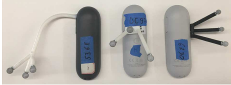
Fig. 1: Different versions of Vicon attachments to controller.
