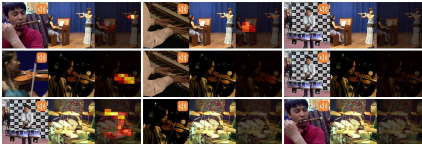
Fig. 6. What would make this sound? Similarly to Figure 5, the AVOL-Net localization output is shown given an input image frame and 1s of audio. However, here the frame and audio are mismatched. Each triplet of images shows the (left) input audio, (middle) input frame, and (right) localization output overlaid over the frame. Purely for visualization purposes, as it is hard to display sound, the frame of the video that is aligned with the sound is shown instead of the actual sound form (left). On the example of the first triplet: (left) flute sound illustrated by an image of a flute, (middle) image of a piano and a flute, (right) the flute from the middle image is highlighted as our network successfully answers the question “What in the piano-flute image would make a flute sound?” In each row the input frame is fixed while the input audio varies, showing that object localization does depend on the sound and therefore our system is not just detecting salient objects in the scene but is achieving the original goal – localizing the object that sounds.
