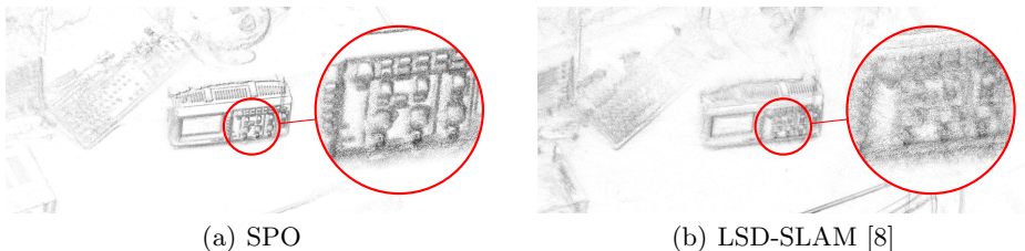
Fig. 9. Point clouds of the same scene: (a) calculated by SPO and (b) calculated by LSD-SLAM. Because of its narrow field of view, the plenoptic camera has much smaller ground sampling distance, which, in turn, results in more detailed 3D map than for the monocular camera. However, as a result the reconstructed map is less complete.
