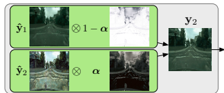
Fig. 4. Illustration of the linear combination in an adaptive fusion block. The fusion block applies the fusion weight map \alpha to find defects in the previous result \hat{y}_1 and correct it precisely using \hat{y}_2 to produce a refined output y_2 .
