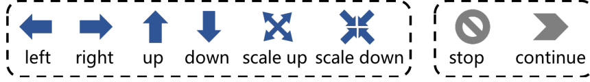
Fig. 4. The defined actions of two agents. Left: movement actions for the tracking agent. Right: stop/continue actions for the alignment agent.
