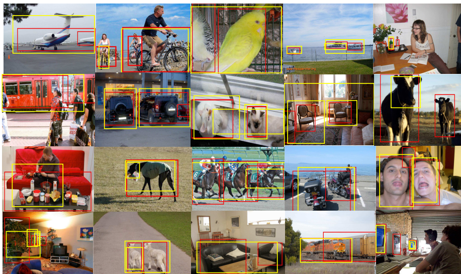
Fig. 8. Qualitative comparison between our CWSL:ODR+FRCNN (red boxes) and OICR+FRCNN (yellow boxes) on the VOC2007 test set over the 20 classes. Our detector detects much tighter bounding boxes, yields much fewer boxes with multiple objects in them, and finds instances more accurately
