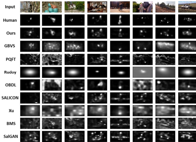
Fig. 6. Saliency maps of 8 videos randomly selected from the test set of our eye-tracking database. The maps were yielded by our and 8 other methods as well the ground-truth human fixations. Note that the results of only one frame are shown for each selected video.
