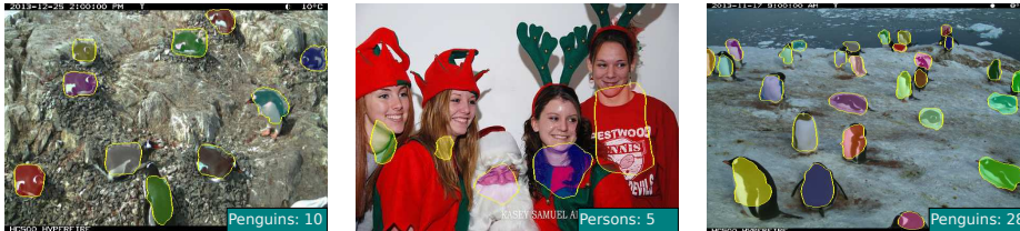
Fig. 1. Qualitative results on the Penguins [1] and PASCAL VOC datasets [2]. Our method explicitly learns to localize object instances using only point-level annotations. The trained model then outputs blobs where each unique color represents a predicted object of interest. Note that the predicted count is simply the number of predicted blobs.
