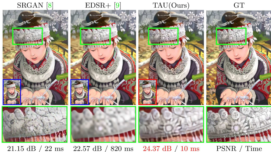
Fig. 1: Our task-aware downsampled (TAD) image (red box) generates more realistic and accurate HR image compared with the state-of-the-art methods that use bicubic-downsampled LR images (blue box). TAD image shows good LR image quality and, when upscaled with our jointly trained upscaling method TAU, outperforms EDSR+ by a large margin with considerably faster runtime. The scaling factor 1 is \times 4 .
