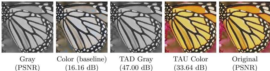
Fig. 6: Qualitative image colorization results. The leftmost image is used as I^{guide} for our model and input grayscale for the baseline. The channel scale factor \times 3 .
