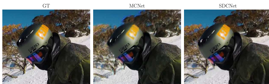
Fig. 1. Frame prediction on a YouTube video frame featuring a panning camera. Left to right: Ground-truth, MCNet [34] result, and our SDC-Net result. The SDC-Net predicted frame is sharper and preserves fine image details, while color distortion and blurriness is seen in the tree and text in MCNet’s predicted frame.
