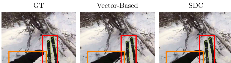
Fig. 10. Comparison of frame synthesis operations. Ground-truth frame (left), Vector-based sampling (middle), and SDC (right). Some foreground duplication (orange box) and inconsistent pixel synthesis (red box, may require zooming in) are present in the Vector-based approach but resolved in the SDC results.
