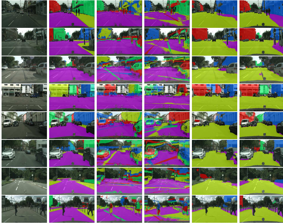
Fig. 6. Plane segmentation results on Cityscapes. From left to right: Input image; Ground truth; Depth + J-Linkage; Depth + Ransacov; Ours (w/o fine-tuning); Ours (w/ fine-tuning).
