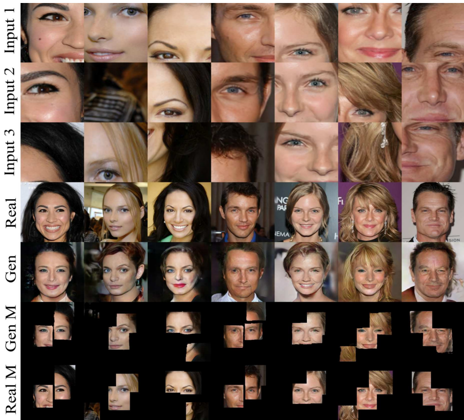
Fig. 6. Generated images and predicted masks on the CelebA-HQ dataset. Three key local patches (Input 1, Input 2, and Input 3) are from a real image (Real). Given inputs, images and masks are generated. We present masked generated images (Gen M) and masked ground truth images (Real M).
