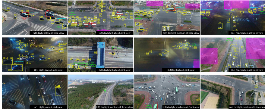
Fig. 1. Examples of annotated frames in the UAVDT benchmark. The three rows indicate the DET, MOT and SOT task, respectively. The shooting conditions of UAVs are presented in the lower right corner. The pink areas are ignored regions in the dataset. Different bounding box colors denote different classes of vehicles. For clarity, we only display some attributes.
