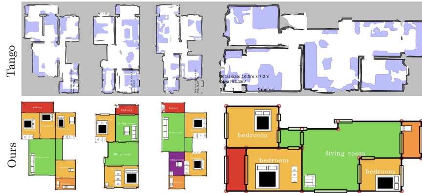
Fig. 7. Comparison against a commercial floorplan generator, Tango Navigator App. Top: Floorplan image from Tango. Bottom: Our results.
