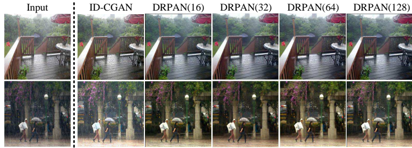
Fig. 6. Example results of our DRPAN with different sizes of discriminative region compared to ID-CGAN [43] on single image de-raining task.
