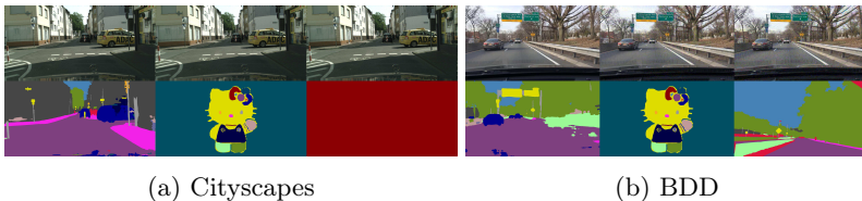
Fig. 2: Samples of benign and adversarial examples generated by Houdini on Cityscapes [11] (targeting on Kitty/Pure) and BDD100K [53] (targeting on Kitty/Scene). We select DRN as our target model here. Within each subfigure, the first column shows benign images and corresponding segmentation results, and the second and third columns show adversarial examples with different adversarial targets.
