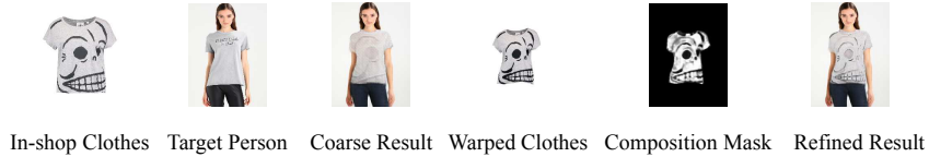
Fig. 6. An example of VITON stage II. The composition mask tends to ignore the details of coarsely aligned clothes.
