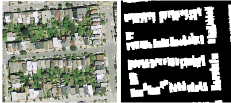
Fig. 2. Multimodal pair of satisfyingly aligned images, from the database. Left: aerial RGB image, right: vector-format cadastral image (buildings are shown in white).
