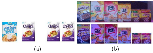
Fig. 6. (a) Reconstruction of Fig. 1(a). (b) Correct reconstruction (bottom row) of shelf image (top row). Product with minor variation (two boxes at the right end) is correctly identified.
