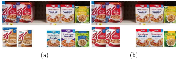
Fig. 10. (a) Winner product at a shelf location is selected based on maximum NSURF score. (b) Result using composite score (top row: original shelf image, bottom row: reconstruction).
