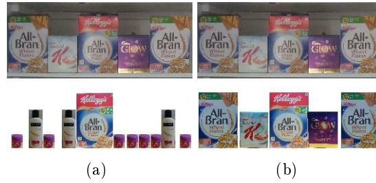
Fig. 9. (a) Winner product at a shelf location is selected based on maximum correlation score. (b) Result using composite score (top row: original shelf image, bottom row: reconstruction).
