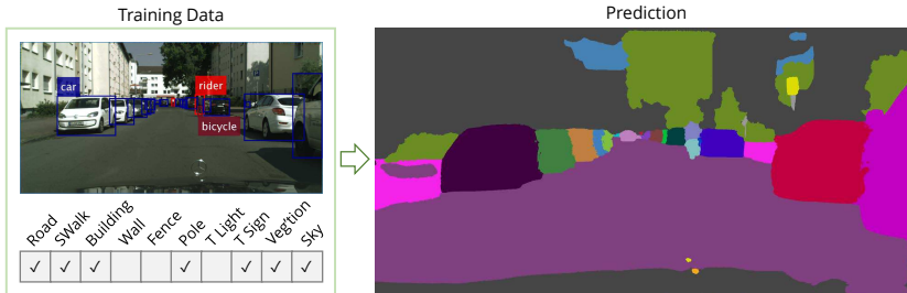
Fig. 1. We propose a method to train an instance segmentation network from weak annotations in the form of bounding-boxes and image-level tags. Our network can explain both “thing” and “stuff” classes in the image, and does not produce overlapping instances as common detector-based approaches [22–24].
