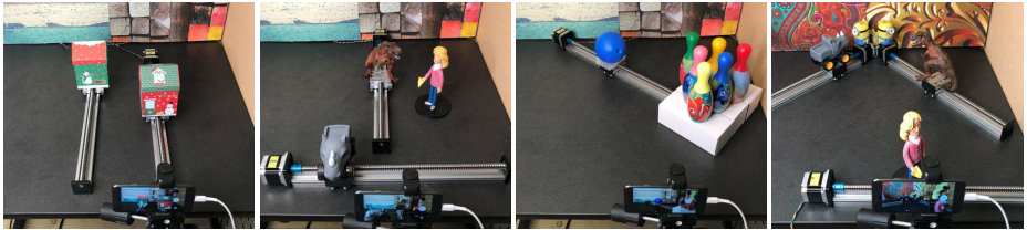
Fig. 2: A top view of our capture environment. Each shoot contains the scene components: linear stage actuators, smartphone camera, tripod, objects, and scene background.
